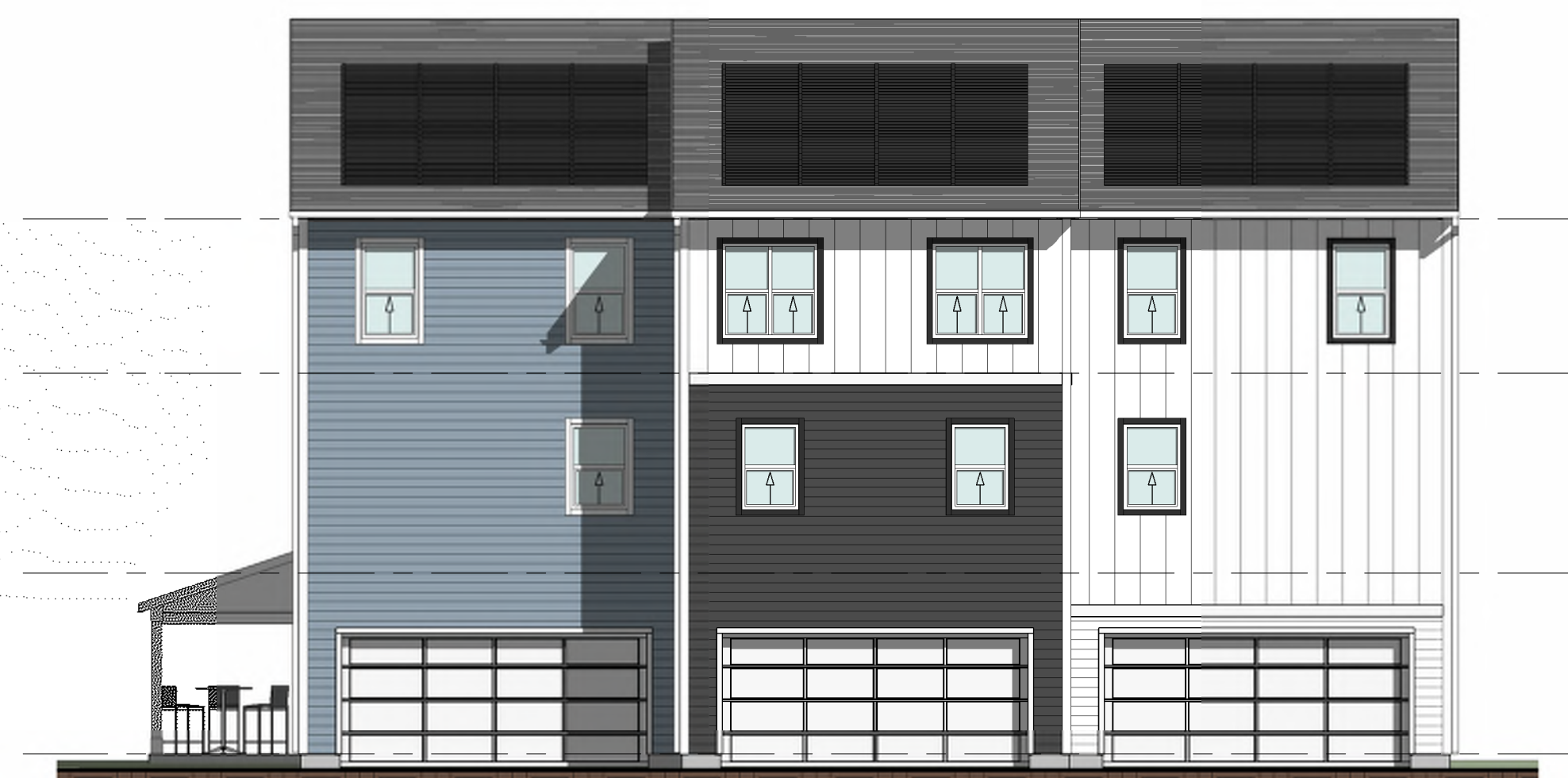
③ REAR ELEVATION - BUILDING H3.0 1/8" = 1'-0" FACADE: 1,700 SQ FT WINDOWS: 178 SQ FT WINDOW PERCENTAGE: 10.5%
