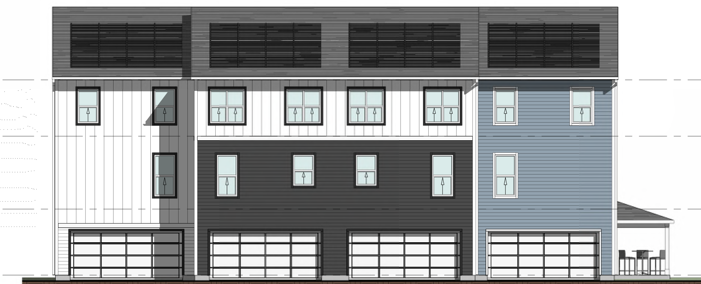
③ REAR ELEVATION - BUILDING H4.1A 1/8" = 1'-0" FACADE: 1,700 SQ FT WINDOWS: 178 SQ FT WINDOW PERCENTAGE: 10.5%
