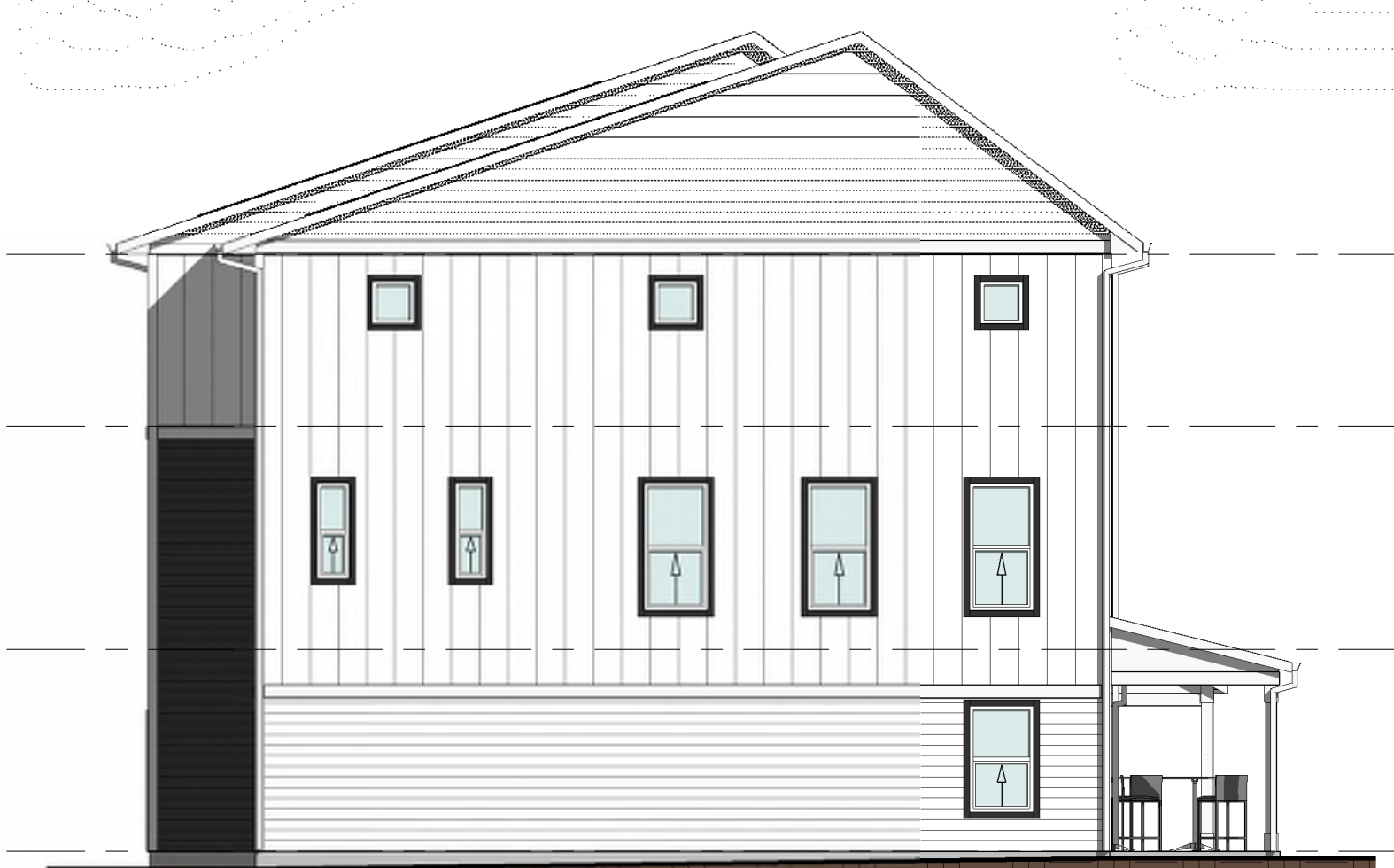
② LEFT ELEVATION - BUILDING H3.0 1/8" = 1'-0" FACADE: 1,367 SQ FT WINDOWS: 147 SQ FT WINDOW PERCENTAGE: 10.8%
