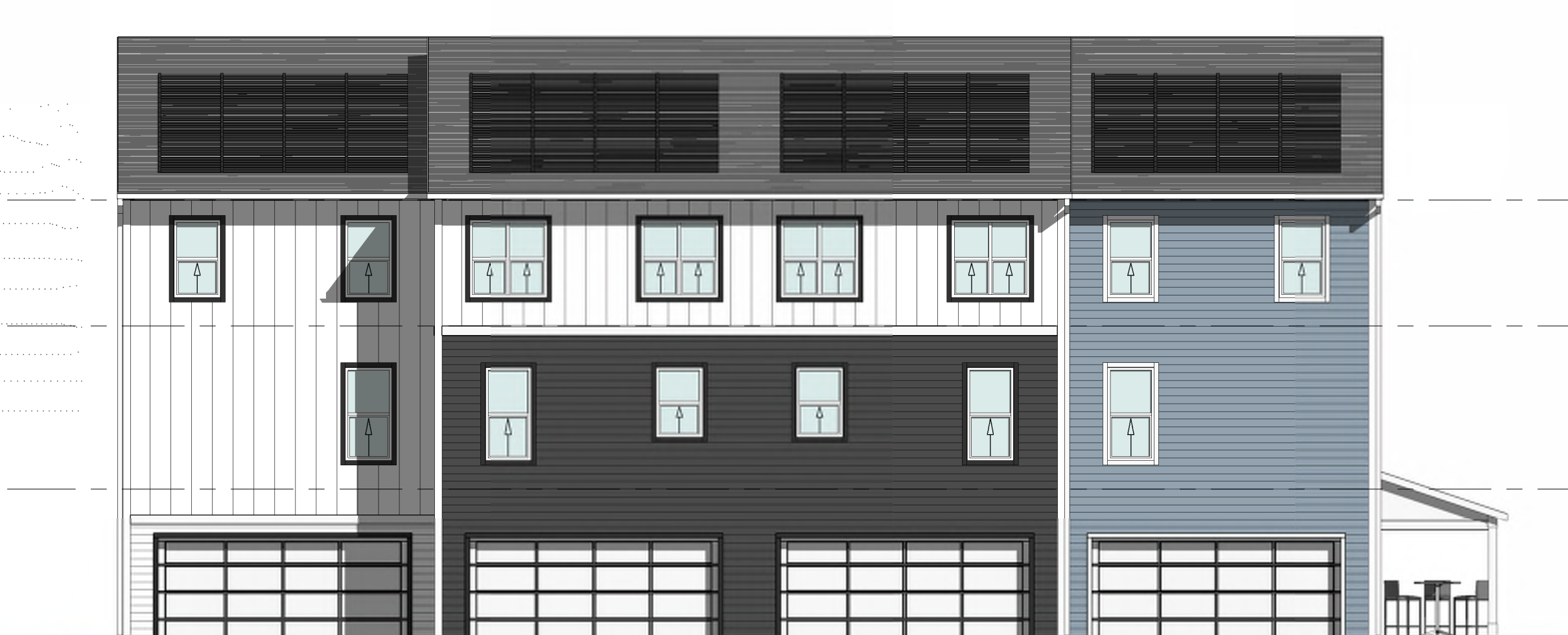
⑦ REAR ELEVATION - BUILDING H4.1B 1/8" = 1'-0" FACADE: 1,700 SQ FT WINDOWS: 178 SQ FT WINDOW PERCENTAGE: 10.5%
