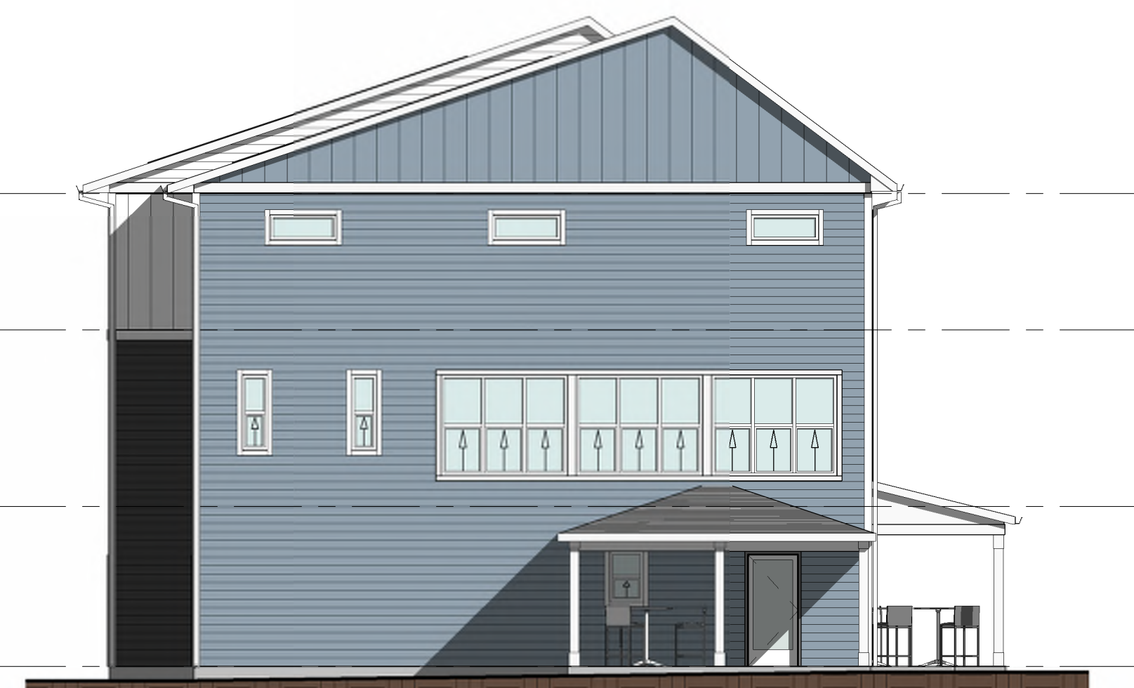
④ LEFT ELEVATION - BUILDING H4.1A 1/8" = 1'-0" FACADE: 1,367 SQ FT WINDOWS: 210 SQ FT WINDOW PERCENTAGE: 15.4%
