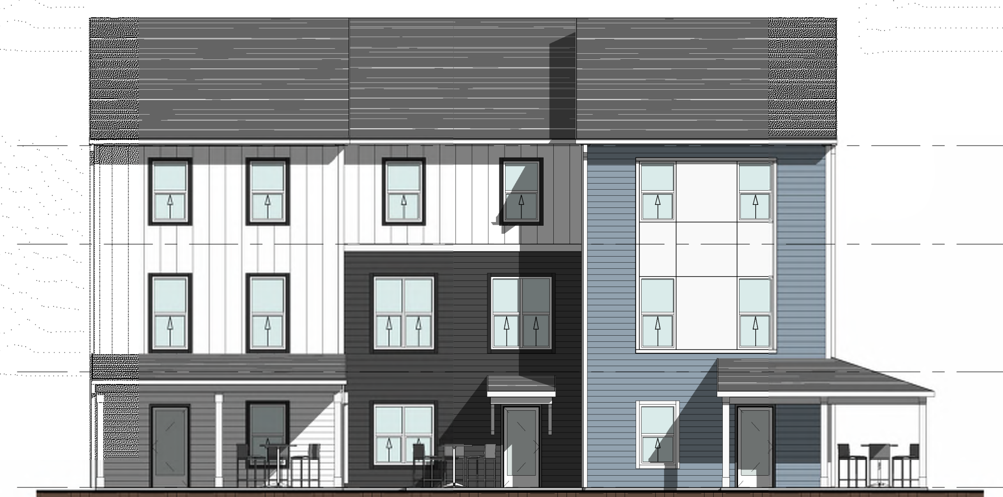
① FRONT ELEVATION - BUILDING H3.0 1/8" = 1'-0" FACADE: 1,700 SQ FT WINDOWS: 277 SQ FT WINDOW PERCENTAGE: 16.3%
