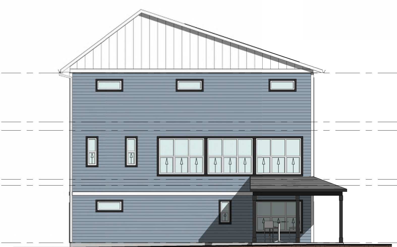
⑧ LEFT ELEVATION - BUILDING H3.1 1/8" = 1'-0" FACADE: 1,367 SQ FT WINDOWS: 215 SQ FT WINDOW PERCENTAGE: 15.7%
