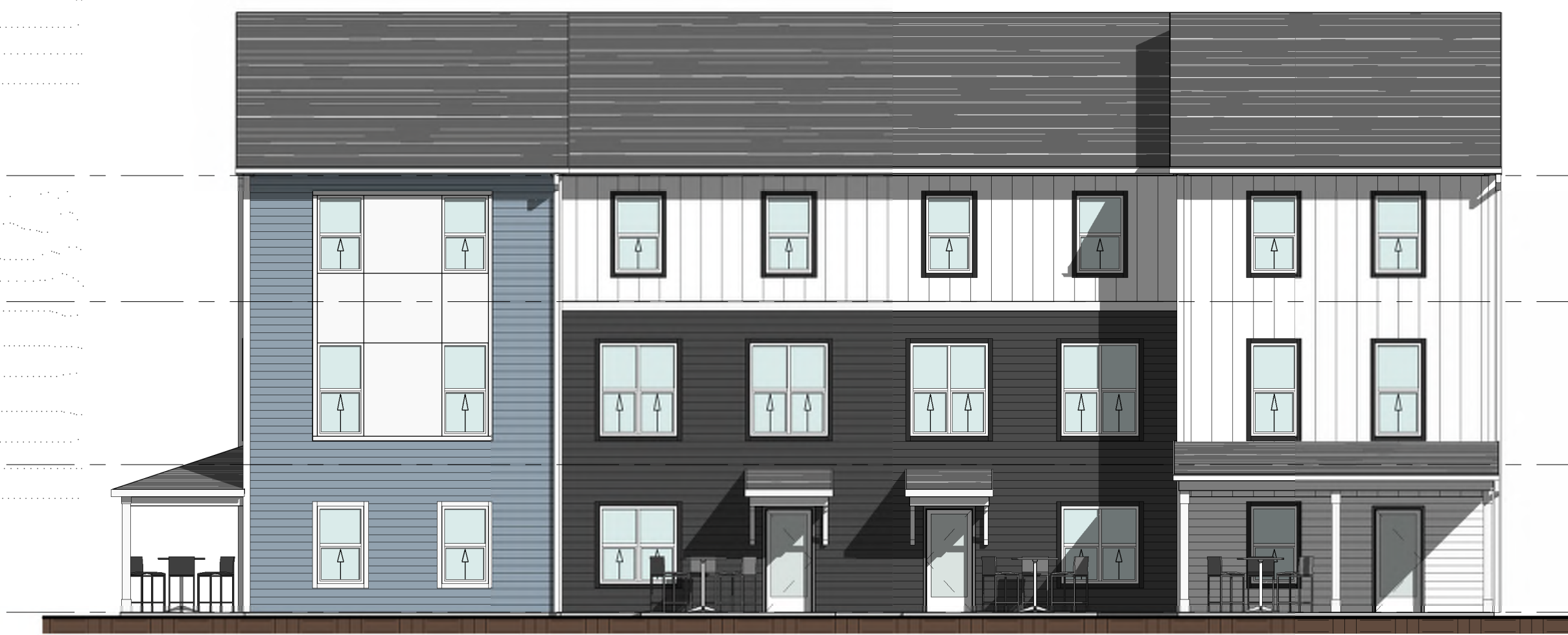
① FRONT ELEVATION - BUILDING H4.1A 1/8" = 1'-0" FACADE: 1,700 SQ FT WINDOWS: 277 SQ FT WINDOW PERCENTAGE: 16.3%
