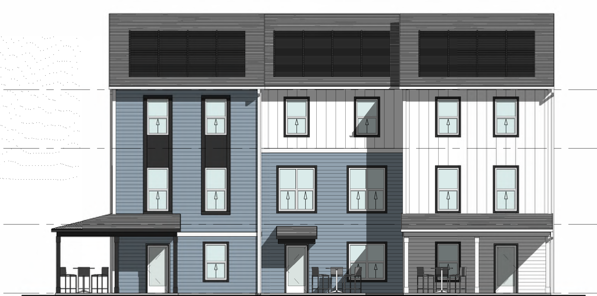
⑤ FRONT ELEVATION - BUILDING H3.1 1/8" = 1'-0" FACADE: 1,700 SQ FT WINDOWS: 277 SQ FT WINDOW PERCENTAGE: 16.3%
