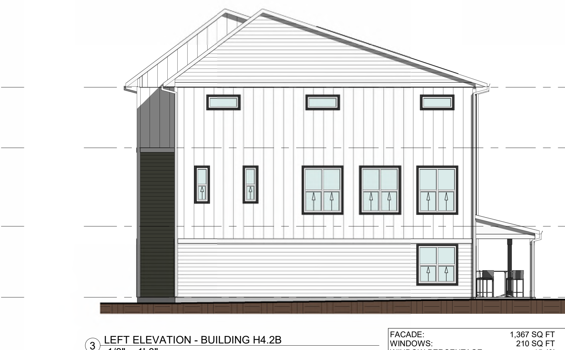
3 LEFT ELEVATION - BUILDING H4.2B 1/8" = 1'-0"
