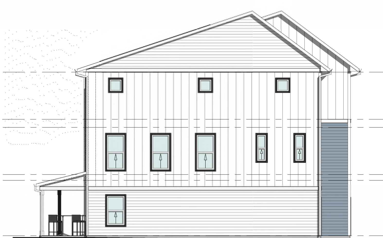
⑥ RIGHT ELEVATION - BUILDING H3.1 1/8" = 1'-0" FACADE: 1,367 SQ FT WINDOWS: 97 SQ FT WINDOW PERCENTAGE: 7.1%
