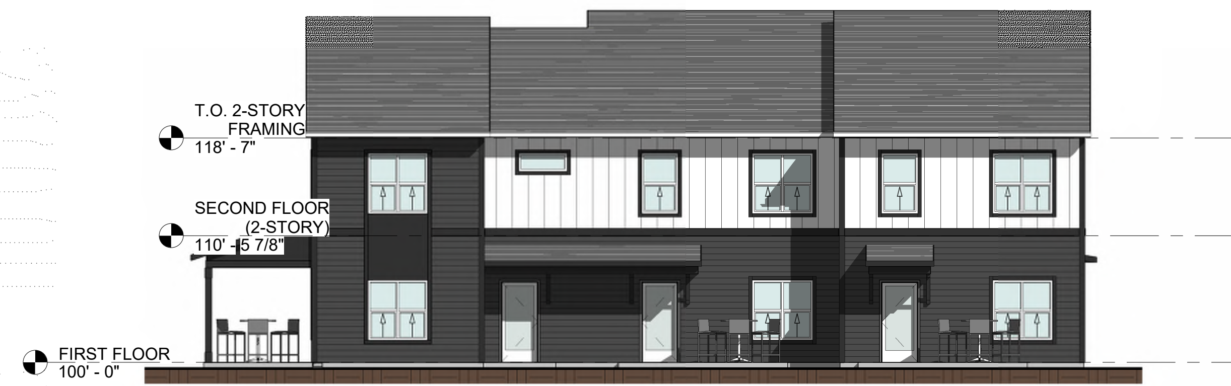
① FRONT ELEVATION - BUILDING W3.0 1/8" = 1'-0"
