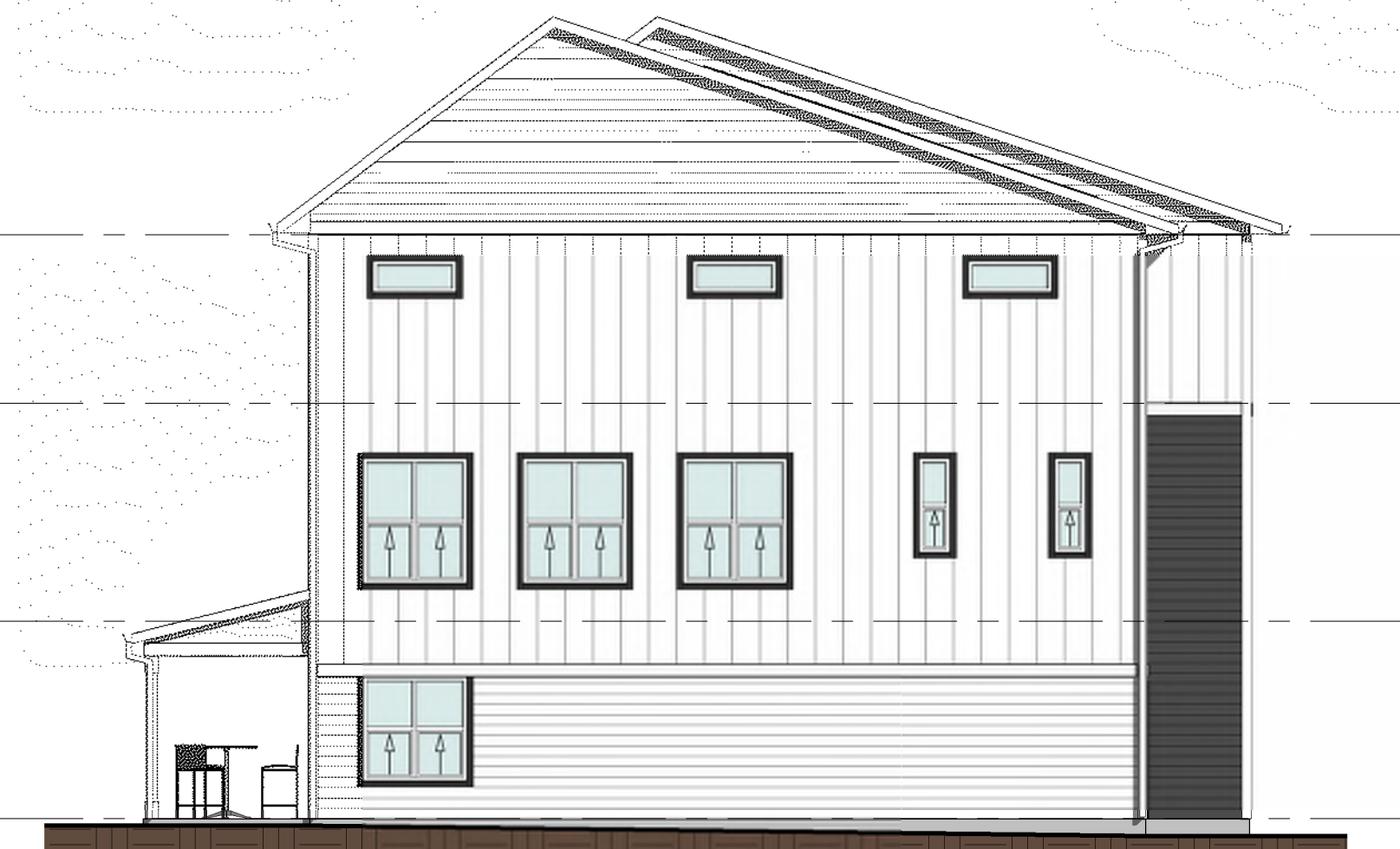
② RIGHT ELEVATION - BUILDING H4.1A 1/8" = 1'-0" FACADE: 1,367 SQ FT WINDOWS: 147 SQ FT WINDOW PERCENTAGE: 10.8%
