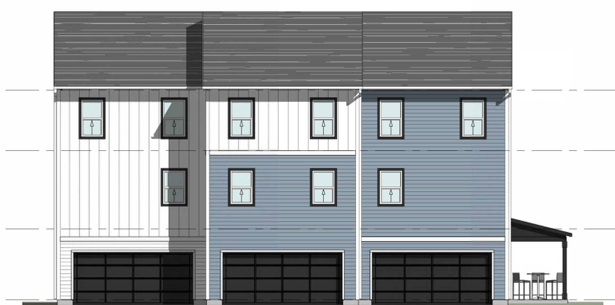
⑦ REAR ELEVATION - BUILDING H3.1 1/8" = 1'-0" FACADE: 1,700 SQ FT WINDOWS: 144 SQ FT WINDOW PERCENTAGE: 8.5%
