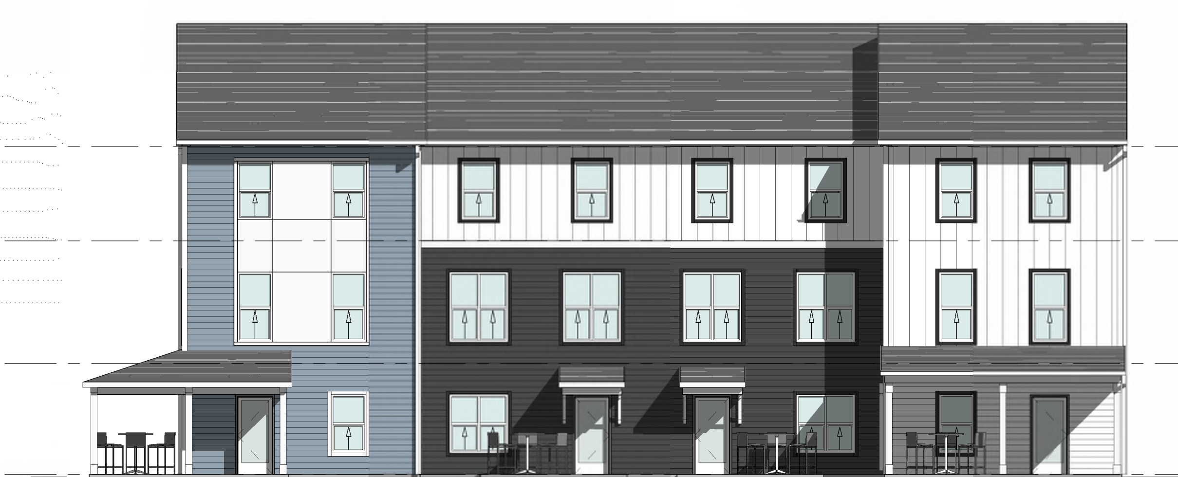
⑤ FRONT ELEVATION - BUILDING H4.1B 1/8" = 1'-0" FACADE: 1,700 SQ FT WINDOWS: 277 SQ FT WINDOW PERCENTAGE: 16.3%
